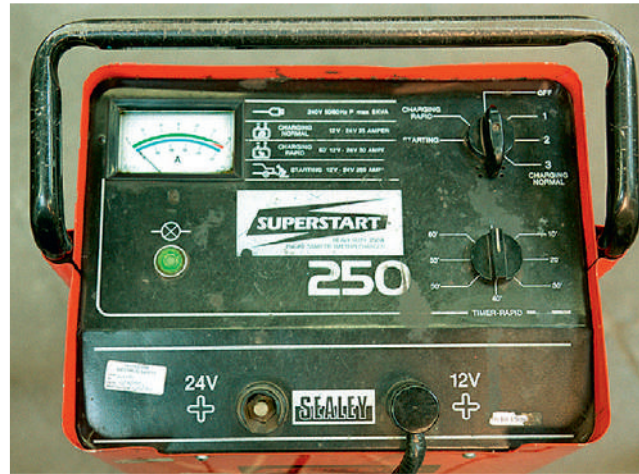
Figure 3.52 Fast charger with time clock
